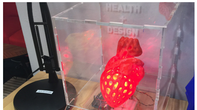
A 3D printed heart model wired with Neopixels and connected to an Arduino powered heart rate monitor to create a heart rate visualizer. Created by: Dr. Robert Pugliese Download and print the model for free: https://www.youmagine.com/designs/anatomical-voronoi-heart
